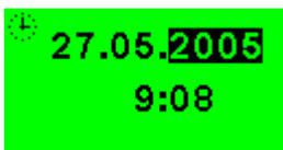
You are now able to adjust the Year, Month, Day, Hour, and Minute. Using the rotary knob, turn clockwise or counter-clockwise to change the highlighted number. Press the rotary knob to proceed to the next number.
