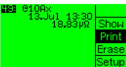
Position the pointer with the rotary knob to highlight “SETUP” and return the RANGE SELECTION screen.
