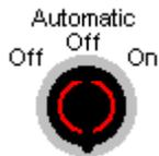
This is the power on switch. Turning the switch to the “ON” position applies power to the test set. Turning the switch to the “OFF” position turns off the instrument. The switch defaults to the “Automatic off” position and will automatically turn off after being idle for a certain period (dependent upon battery charge).
