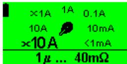
Select the desired test range by turning the rotary knob. The pointer will turn to the available ranges. Press the rotary knob when the desired range is highlighted to select that range.
